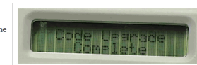
This time-lapsed image of a screen on an HP LaserJet shows the impact of a rogue print job used to reprogram the device.
