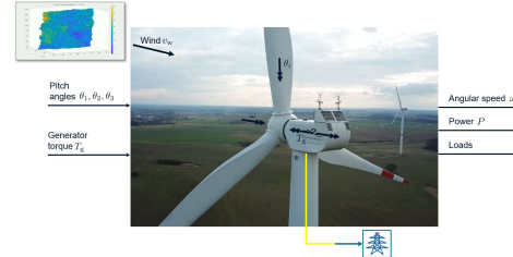
Wind Turbine Control is Speed and Power Control, and Load Reduction
