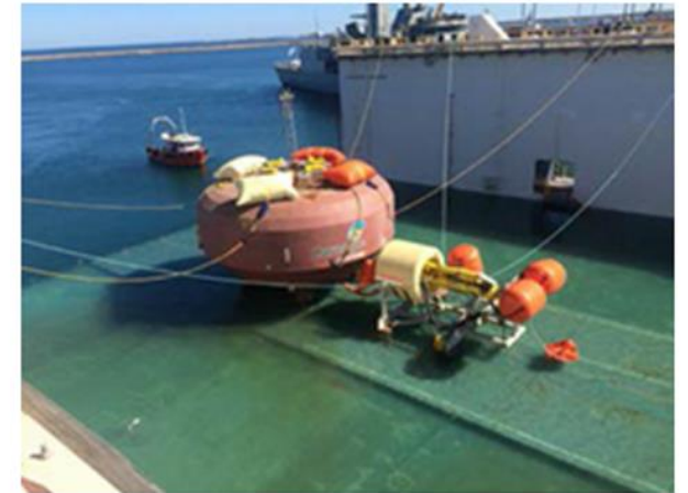
A CETO unit ready for deployment in the wave farm.
