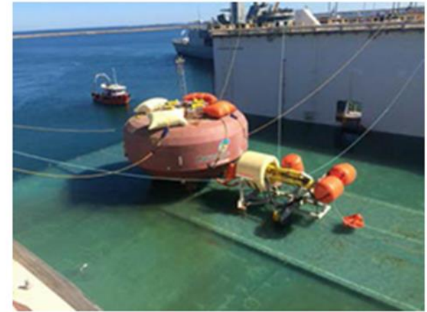
A CETO unit ready for deployment in the wave farm.
